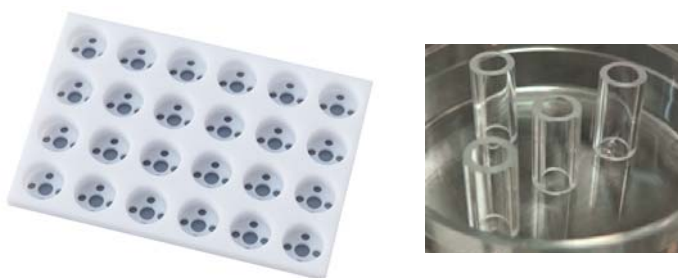
Figure 1. CellSpotter-comfort24(left) and cloning rings (right). Cells will be amounted onto the recording electrodes through cloning rings placed in the center-hole of the CellSpotter.
